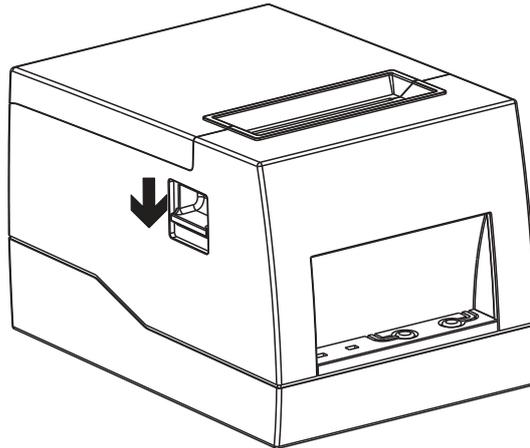
2. Hold the printer and lift up the paper roll spindle and the paper roll stopper.
