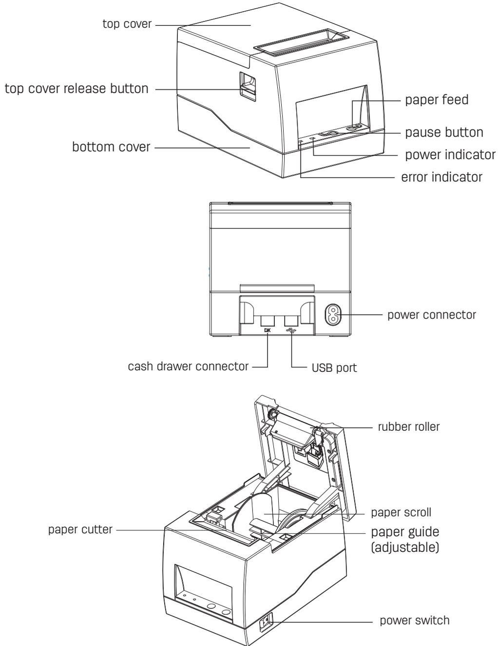
Note: Keep your fingers away from the paper cutter while printing, or you may cut your finger. The company shall not be liable for any injury caused by the paper cutter during operation.
